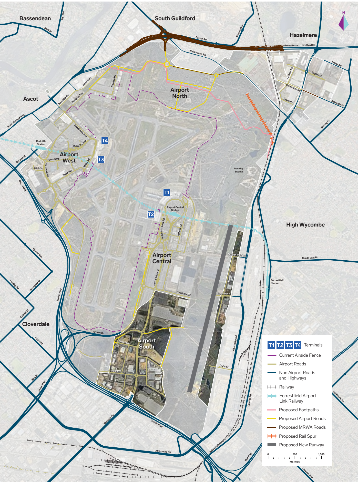
Figure 6-11 Five-year ground transport plan concept for Airport South (Road layout to be confirmed during MDP development) Source: Perth Airport
