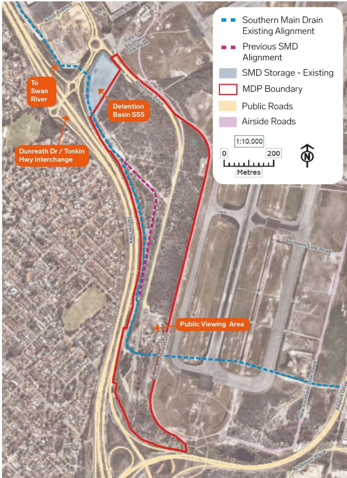
Figure 6-2 Existing Stormwater Management Conditions across Airport West (South) project site
